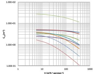
S3-1. Relationship between virus number concentration for each droplet size,  $C_{v,d}$  ( $n_0=10^6 \text{ mL}^{-1}$ ) and ventilation rate. The droplet size  $d_0$  is the initial one before shrinkage.
