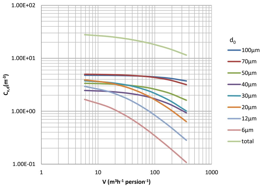
**S3-2 - Relationship between droplet mass concentration for each initial size,  $C_{m,d}$  and ventilation rate** The droplet size  $d_0$  is the initial one before shrinkage.
