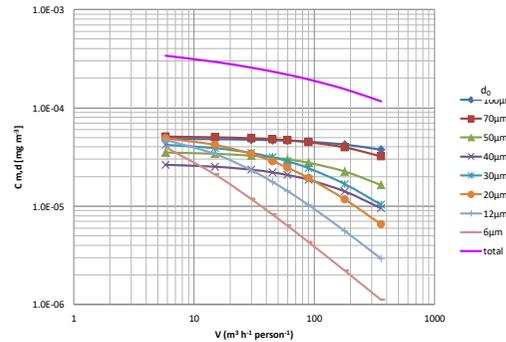
S3-2. Relationship between droplet mass concentration for each initial size and ventilation rate. ( $\lambda=0$ )
